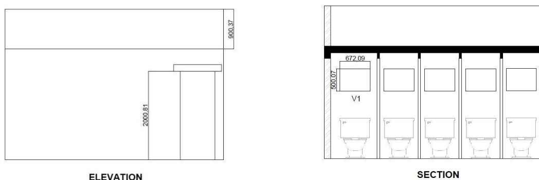
Figure 58 Elevation & section of Public Toilet
